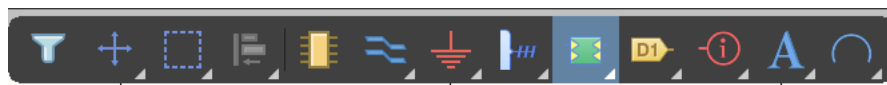
Figure 21: Screenshot showing the location of the sheet symbol tool on the upper toolbar
