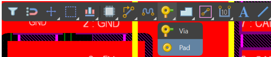
Figure 49: Screenshot showing how to access the pad tool from the upper toolbar
