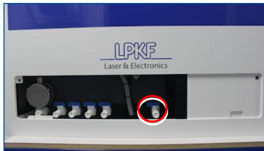
Fig. 54: Drain valve of tank 6
