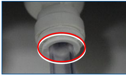
Fig. 55: Ring on drain valve
