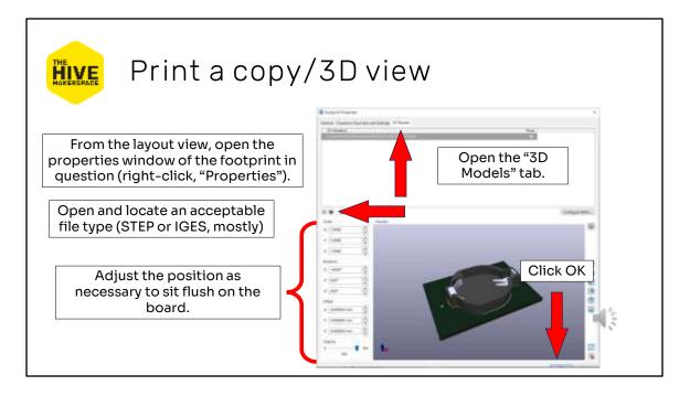
A well-designed 3D CAD model should have the origin aligned properly such that one or two rotations should have the part sitting flush, if that.
