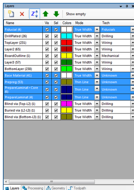
Fig. 101: Pane Layers and highlighted auxiliary layers.
