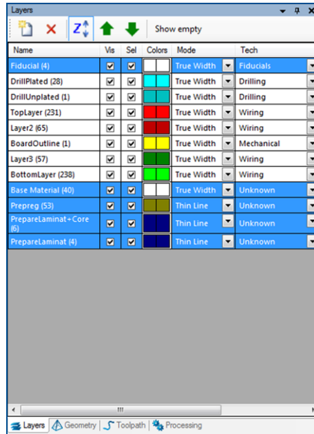
Fig. 85: Pane Layers and highlighted auxiliary layers
