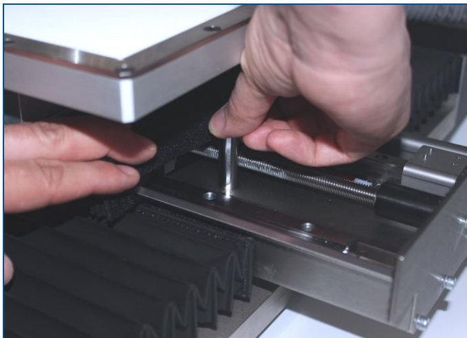
Fig. 45: Pulling out the bolt
